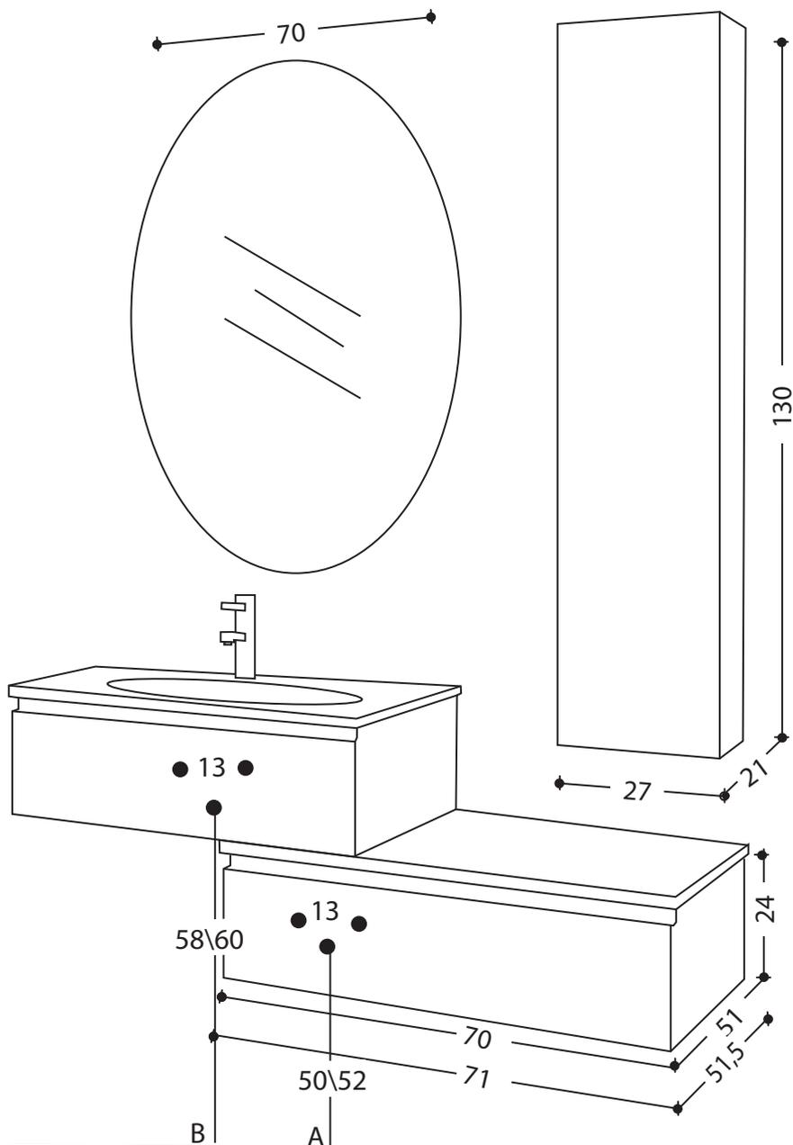
A: SE IL SIFONE PASSA NEL MOBILE SOTTO - PREVEDERE SCARICO A H 50\52
